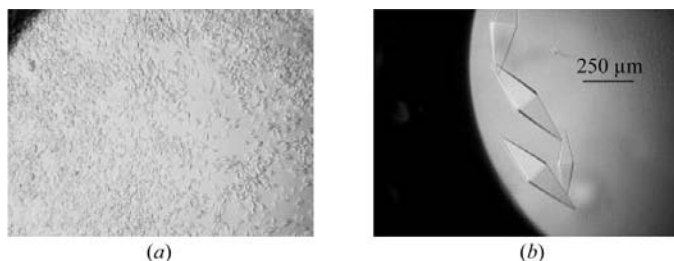
Figure 3 Optimization of Pfu-1862794 using response-surface methodology (RSM) and central composite design (CCD). (a) Conditions that produced micro-crystals obtained during coarse screening (288 conditions). (b) Crystals produced from the RSM/CCD-predicted conditions based on 13 RSM/CCD experiments. Images were recorded using the DeCode Genetics imaging system supplied with Crystal Monitor.
